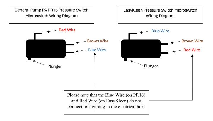
The microswitch is located inside the housing of the pressure switch. The General Pump PA PR16's microswitch is connected differently than the original one from EasyKleen. They wire to the same place in the electrical box, it's just that the wiring colors attached to the microswitch are connected in different areas. See the above diagram for each switch.
